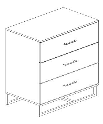
It is recommended that you fit the anti-tip bracket to this item to avoid tipping and causing injury.
